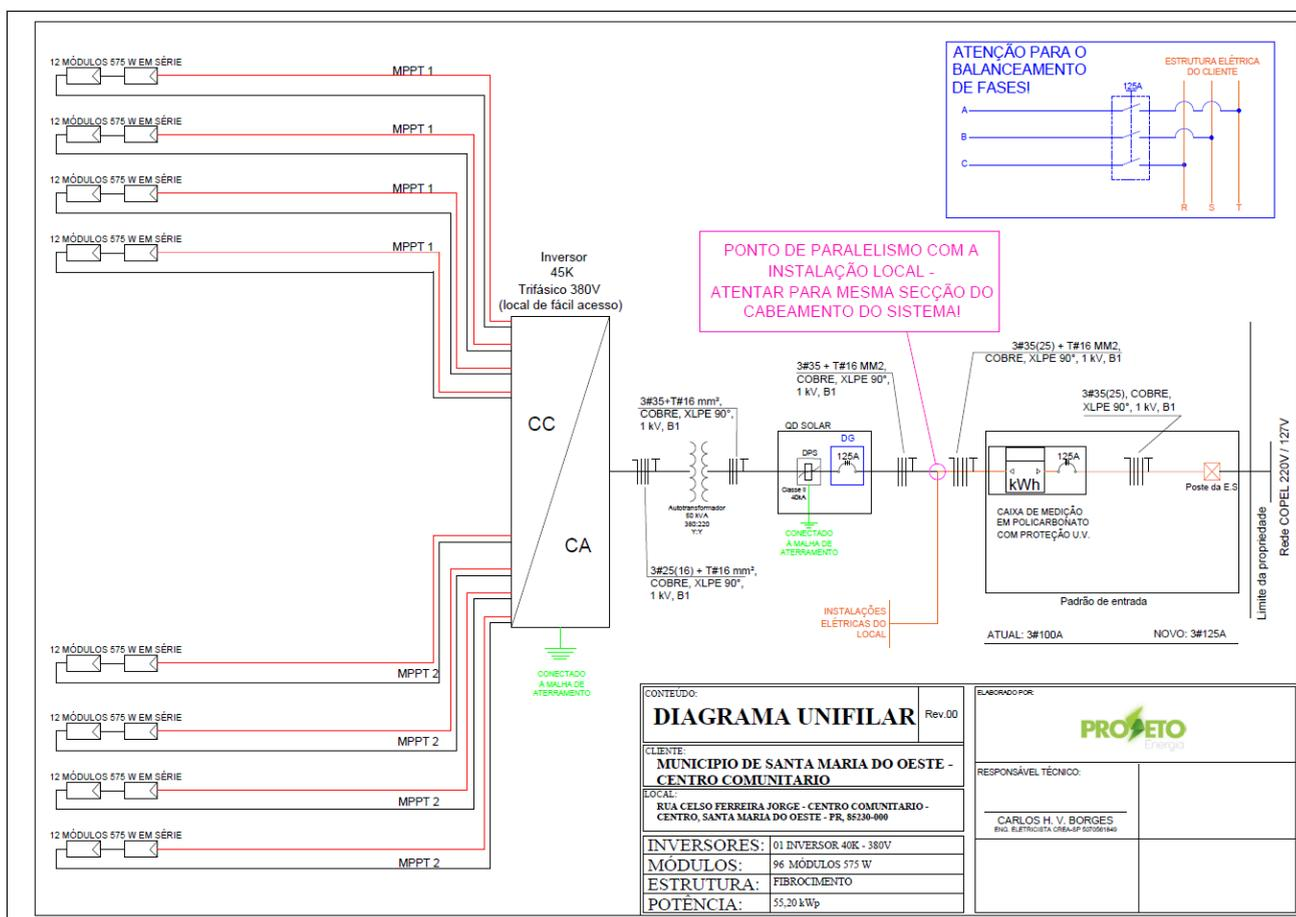
Figura 28 - Diagrama unifilar Local (4)
